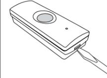
Insert a flathead screwdriver into the slot below the battery and gently prise to remove. Insert 1 x CR2032 button cell battery, ensuring it is positive (+) side up.
