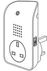
Within 30 seconds of the double "beep" press the button on the front of the bell push. The chime will sound.
