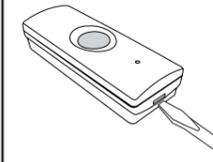
Insert a flathead screwdriver into the slot below the battery and gently prise to remove. Insert 1 x CR2032 button cell battery, ensuring it is positive (+) side up.
