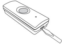
Press the black button marked "S" inside the bell push. Each time you press the button it will play a different chime sound. Stop when you hear the one you want.
